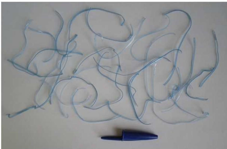
**Fig. 4.** Fibres obtained from waste PET bottles.
