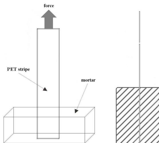
Fig. 6. The concept of testing adhesion of PET to the cement matrix.
