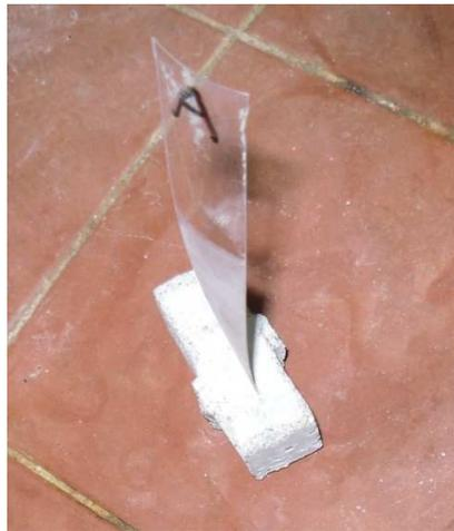
Fig. 5. Specimen for testing adhesion of the PET stripe to the cement matrix.
