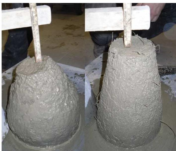
**Fig. 7.** Slump test for the concrete mix without PET fibres (left) and with 0.1% (by volume) PET fibre (right).
