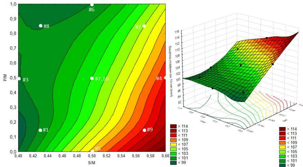
**Fig. 6.** Consistency of polymer concrete mix tested according to flow table procedure (10 minutes after mixing) vs. the material variables  $x_1 = B/M$  (polymer binder to microfiller mass ratio),  $x_2 = P/M$  (waste powder to microfiller mass ratio).
