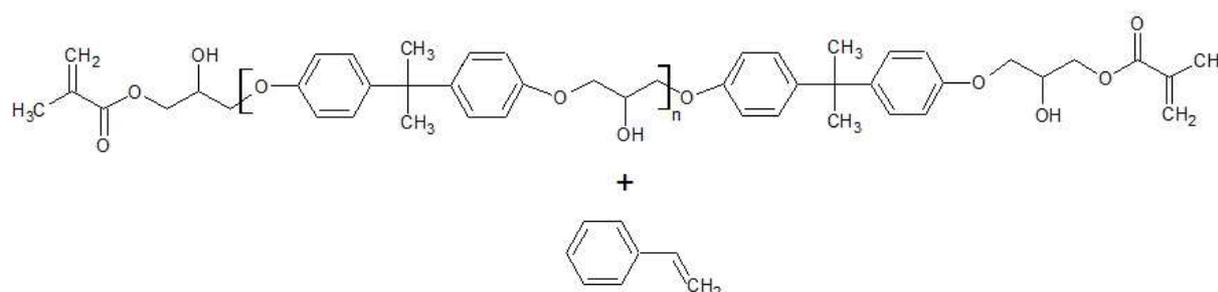
Fig. 1. Vinyl-ester resin (used as the binder in tested composites) before cross-linking.
