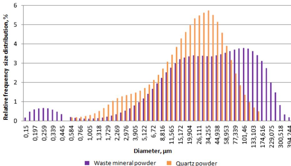
**Fig. 3.** Relative frequency of grain size distribution of waste powder and quartz powder.
