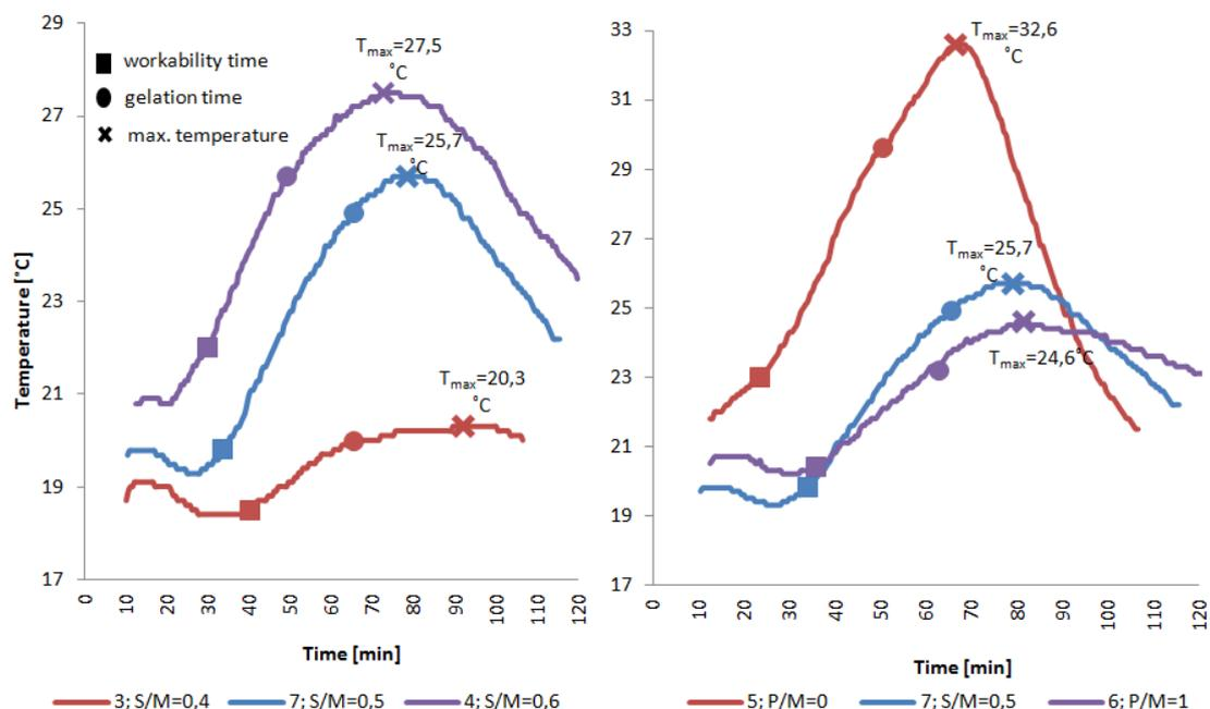
**Fig. 4.** Temperature in time of setting of vinyl-ester micro-mortars of various content of polymer but the same proportion of quartz and waste powders in microfiller: P/M = 0.5 (left) and different proportions of powders but constant polymer to microfiller ratio B/M = 0.5 (right).
