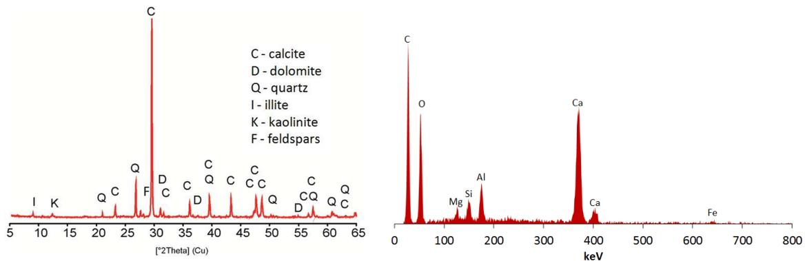
**Fig. 2.** Composition mineral powder: X-ray powder diffractogram (left), energy dispersive spectrum (right) – the detected components confirm the conformity with the aggregate the waste is derived from.
