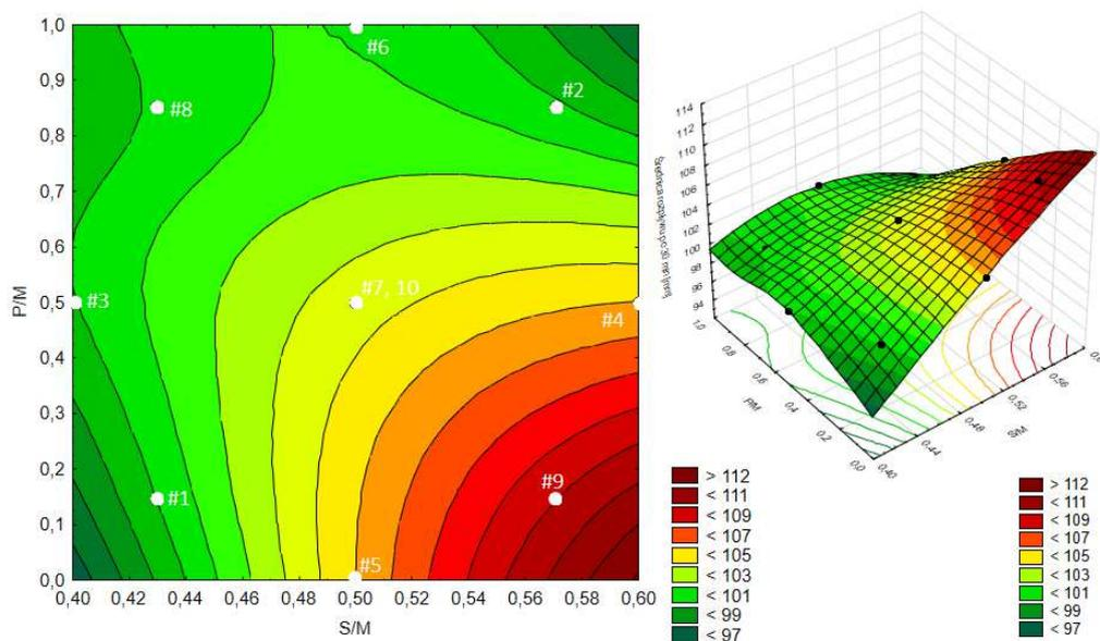
**Fig. 7.** Consistency of polymer concrete mix tested according to flow table procedure (30 minutes after mixing) vs. the material variables  $x_1 = B/M$  (polymer binder to microfiller mass ratio),  $x_2 = P/M$  (waste powder to microfiller mass ratio).
