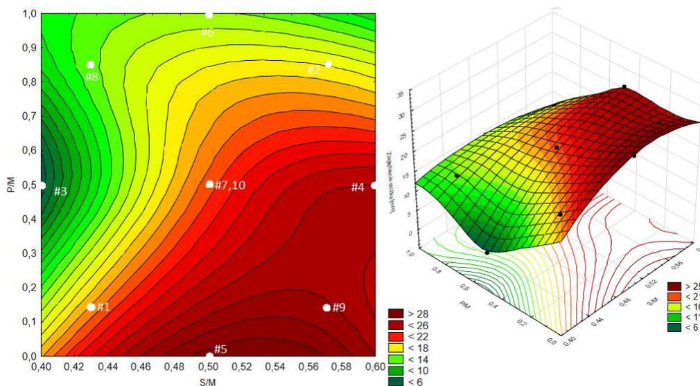
**Fig. 5.** Consistence of polymer concrete mix tested according to cone penetration procedure (10 minutes after mixing) vs. the material variables  $x_1 = B/M$  (polymer binder to microfiller mass ratio),  $x_2 = P/M$  (waste powder to microfiller mass ratio).
