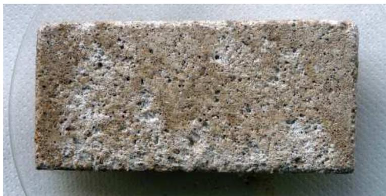
**Fig. 5.** Sample after five weeks of exposure in salts solution and after drying.
