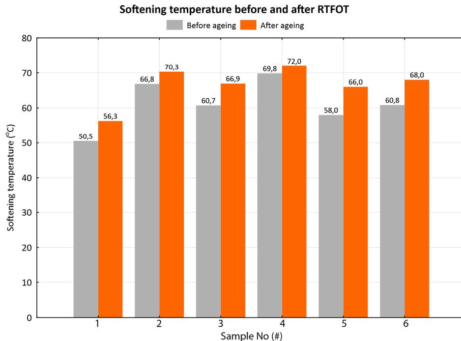
Fig 3. Softening temperature before and after gaining using RTFOT.
