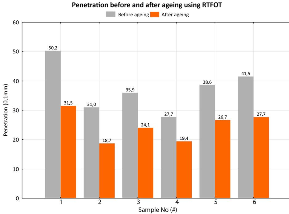
Fig. 2. Penetration before and after gaining using RTFOT.
