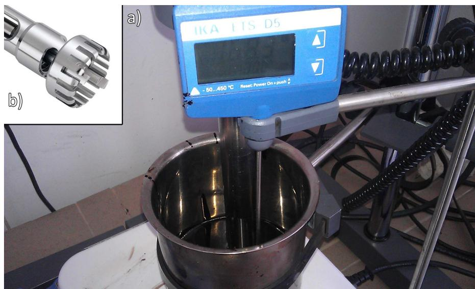
Fig. 1. a) Bitumen modification setup; b) High-shear mixing head.
